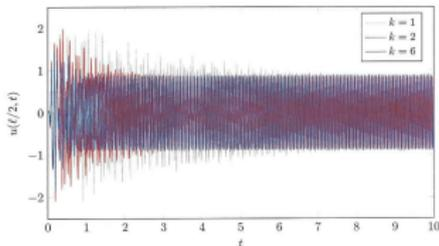
FIGURE 16. Plot of  $u$  at beam midpoint for  $U = 5000$ ,  $b = 20$ ,  $b_0 = 1$ , nonlinear model, varying  $k$ .
