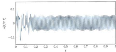
FIGURE 17. Plot of  $u$  at beam midpoint for  $U = 5000$ ,  $b = 5000$ ,  $b_0 = 5000$ ,  $k = 101$  nonlinear model.
